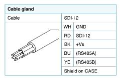
The RS485 interface has not been activated and is to be understood as a factory-installed interface.
