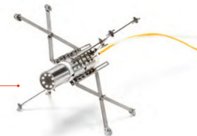
Horizontal centering device for horizontal use - with regulation Ø105-332mm Protects the camera head from accidental shocks and keeps it centered in the hole
