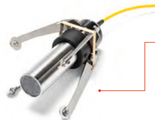
Vertical centering device Ø80-260mm Protects the camera head from accidental shocks and keeps it centered in the hole (other diameter ranges on request)
